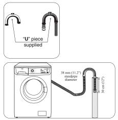
Firstly form a hook in the end of the drain hose using the «U» piece supplied. Place the drain hose into your standpipe, which should have an internal diameter of approximately 38mm thus ensuring there is an air break between the drain hose and standpipe. When discharging into a standpipe ensure that the top of the standpipe is no more than 90 cm (35.4") and no less than 60 cm (23.6") above floor level.
